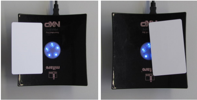
Fig. 11. Exemplary positions of the transponder card on the reader for radiation of higher order harmonics into the far field
