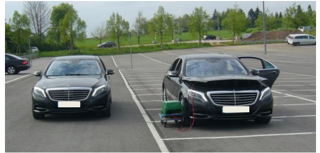
Figure 7: Photo of two Mercedes S-class cars with IR reflecting glass during the measurement
