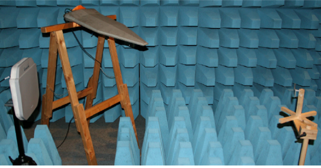
Fig. 4: Measuring setup for which the SIR can be calculated. Reference dipole was replaced by different RFID transponders.
